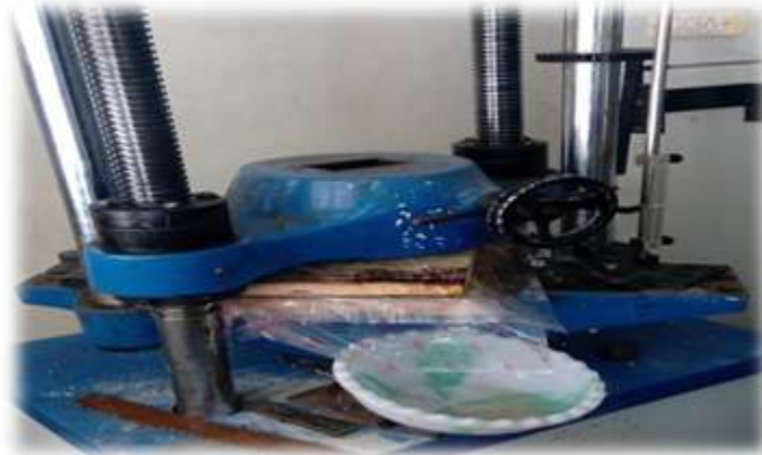
Fig. 4. Compression of Stacking of Fibre Laminates
